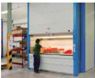
Kardex: automated high-capacity storage system.
