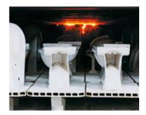
Dried and glazed semi-products are fired at a maximum temperature of 1240 °C.
